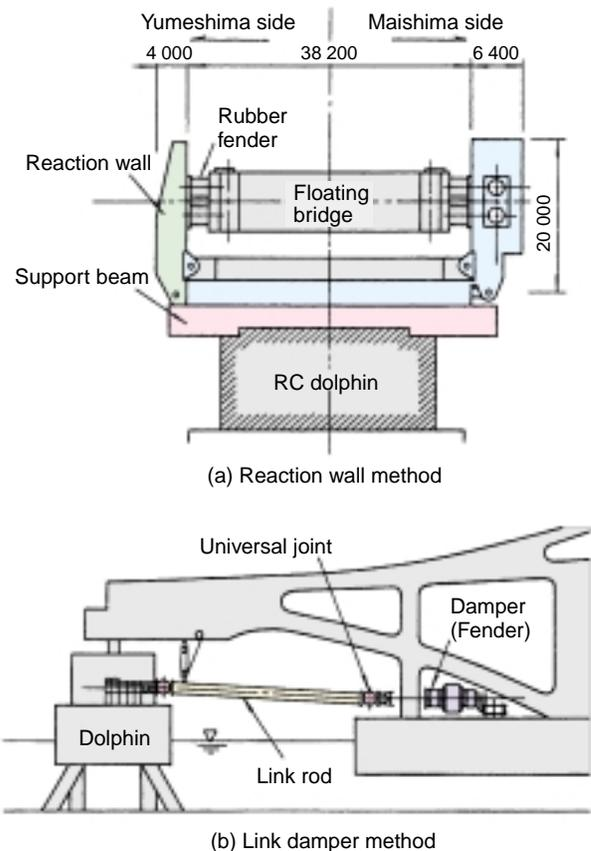
Fig. 6 Schematic of Mooring Systems
