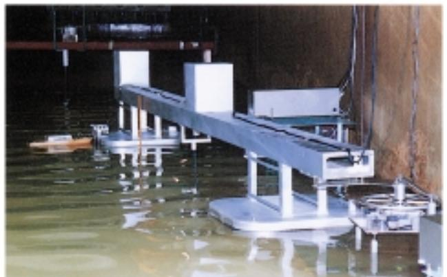
Photo 5 Experiment in Swinging and Temporary Mooring Operations
