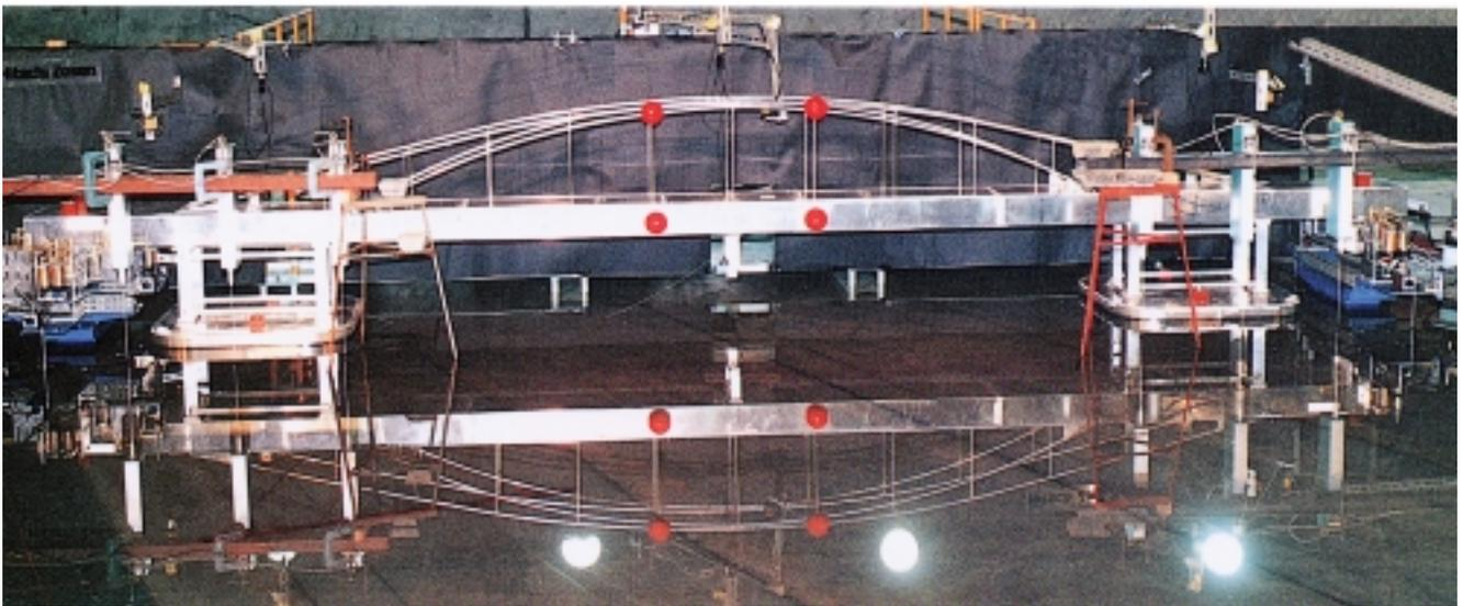
Photo 3 Rigid Model Experiment on In-wave Motion of Moored Floating Structure
